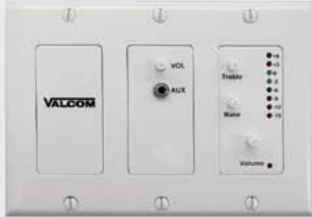
In-Wall Modular Mixer.....V-9983-W - 1 Mounts in 3 Gang Electrical Box • 5.0"W x 4.25"H x 2.0"D (12.7cm x 10.8cm x 5.08cm) 4 lbs (1.5 kg)
